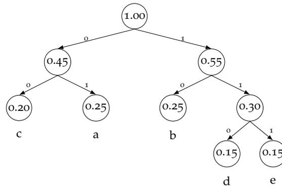
Figure 9: Huffman tree for the example probabilities ( $P(a) = 0.25$ ,  $P(b) = 0.25$ ,  $P(c) = 0.2$ ,  $P(d) = 0.15$ ,  $P(e) = 0.15$ ). The resulting codes (0 for left, 1 for right) are:  $C(a) = 01$ ,  $C(b) = 10$ ,  $C(c) = 00$ ,  $C(d) = 110$ ,  $C(e) = 111$ .
