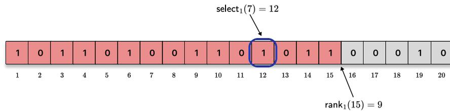
Figure 10: Example of a bitvector  $B[1..20]$ . The prefix  $B[1..15]$  (shaded red) contains 9 ones, so  $\text{rank}_1(15) = 9$ . The 7th 1 (circled blue) occurs at index 12, so  $\text{select}_1(7) = 12$ .
