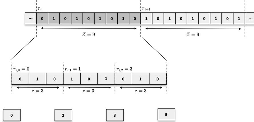
Figure 11: The hierarchical rank data structure. The first level is composed of superblocks of size  $Z$  (storing absolute ranks  $r_i$ ), the second level of blocks of size  $z$  (storing relative ranks  $r_{i,j}$ ), and the third level uses a lookup table (represented by the bottom row).
