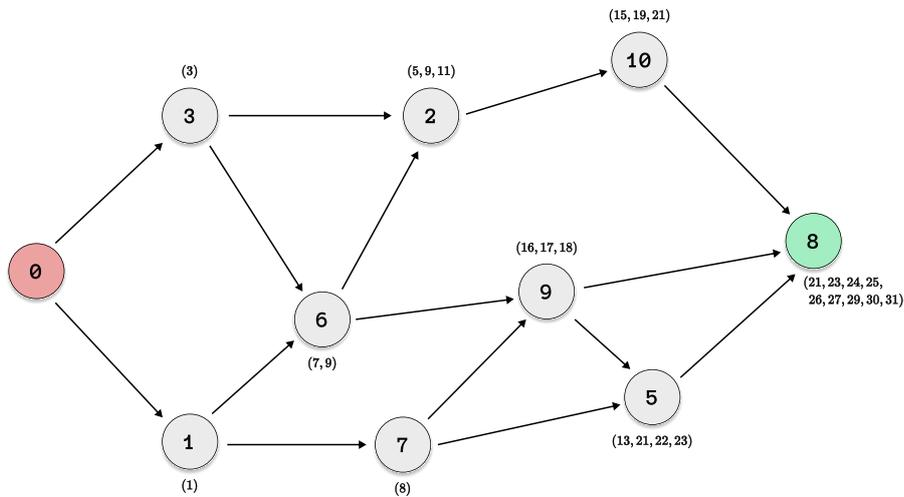
Figure 17: Example of a node-weighted DAG. Each node  $v$  contains its weight  $w(v)$ . The label associated with each node represents its calculated  $\mathcal{O}$ -set,  $\mathcal{O}_v$ , considered as a sorted sequence.
